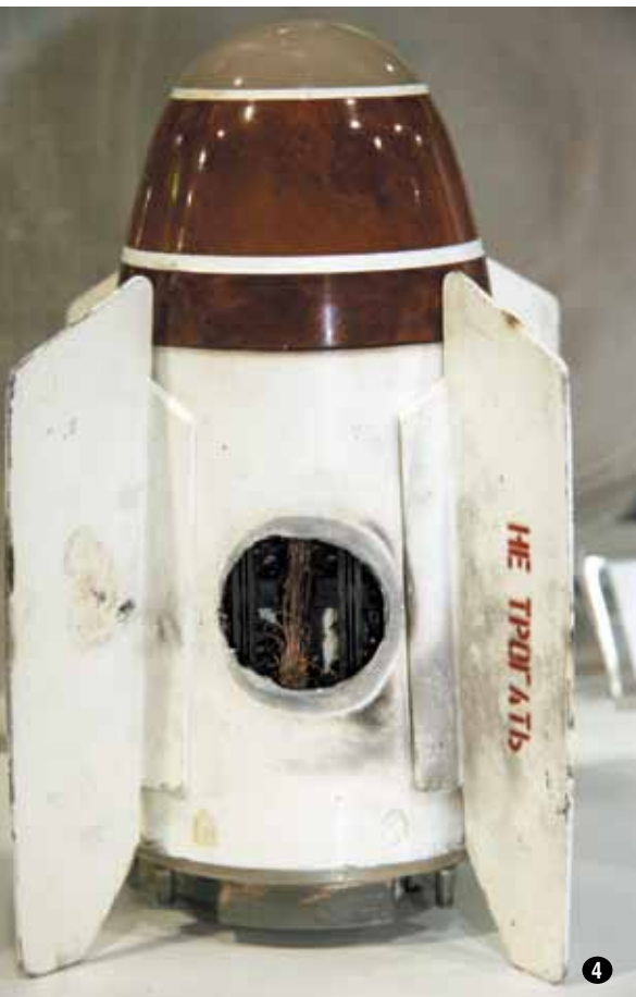
131 Mick Guthals of Textron demonstrates the BattleHawk squad-level loitering munition to CMSgt. Brian Hornback, command chief for Air Force Global Strike Command. 141 The seeker head of a Russian-made Archer air-to-air missile shows the effects of an energy beam fired in a test. AFRL showed a number of artifacts from tests of directed energy weapons.
